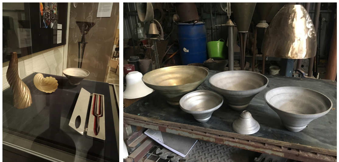
Figure 5 3D printed 'Difference-Tone' bells
